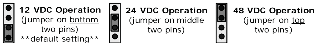
Figure 3-2, DC Voltage Settings
